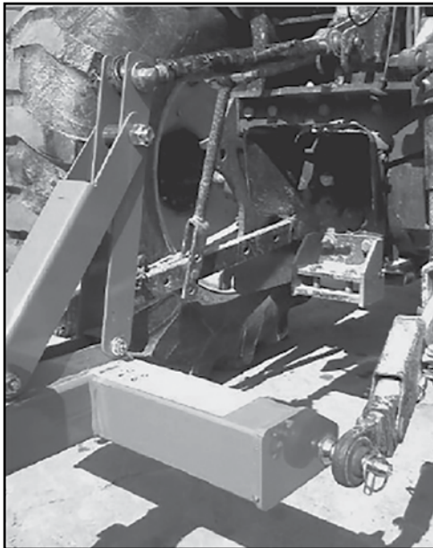
Figure 2. Lower Lift Arm Attachment and Top Link Connection, Category 1
